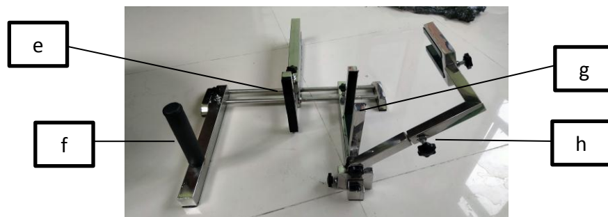
Gambar 4.2 Rancang bangun alat fiksasi Ankle joint Proyeksi Sress View Inversion dan Eversion tampak samping kanan
