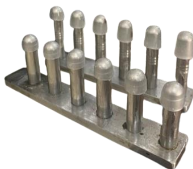
Figure 1. Capsule shell molding process
