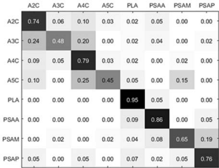
FIGURE 12.26 Confusion matrix of 3D SIFT. The average accuracy is about 73.8%.
