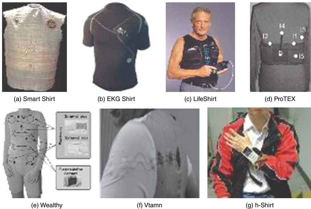
FIGURE 7.10 Various wearable garments for physiological and activity monitoring. (a) The Georgia Tech Wearable Motherboard™ (Smart Shirt) for the measurement of ECG, heart rate, body temperature, and respiration rate [127]; (b) the EKG Shirt system which used interconnection technology based on embroidery of conductive yarn for heart rate [128]; (c) the LifeShirt system for the measurement of ECG, heart rate, posture and activity, respiration parameters, BP (peripheral is needed), temperature, SpO 2 [129]; (d) the ProTEX garment for the measurement of heart rate, breathing rate, body temperature, SpO 2 , position, activity and posture [130]; (e) the WEALTHY system with knitted integrated sensors for the measurement of ECG, heart rate, respiration, activity monitoring [131]; (f) the VTAMN system for the measurement of heart rate, breathing rate, body temperature and activity [132]; (g) the h-Shirt system for the measurement of ECG, PPG, heart rate, and BP [133].
