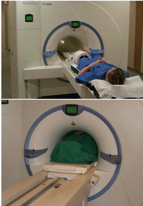
**Fig. 5.1** 7 T MR scanner with a bore of 60cm and a length of 3.50m. The MR is surrounded by 425 tonnes of steel. The *upper figure* shows a person before positioned head first into the scanner. The *second figure* shows a person head first in the scanner with the head in the iso-centre, the feet covered with a sheet
