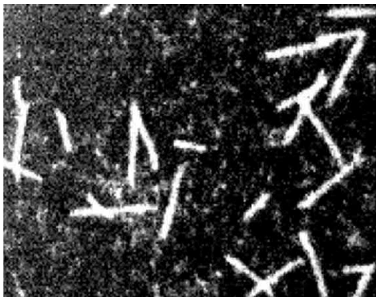
FIGURE 2.23 Superimposed proton–triton tracks obtained with an exposure time of 1 s with a CCD readout of a gas electron multiplier–based neutron detector. From Fraga et al. (2002) , reprinted with permission from Elsevier © 2002.
