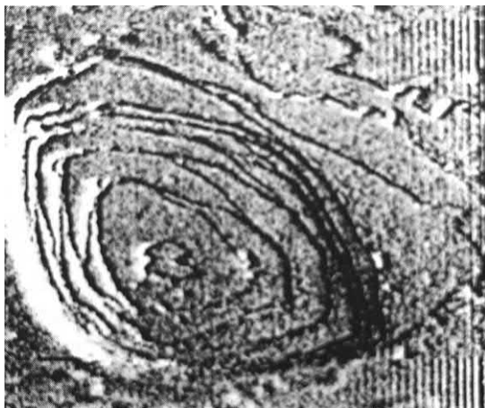
FIG. 3.43 Photograph of an etchpit of a 200 keV Ag track in muscovite mica. The black lines are etched steps bit by the HF etchant. The central part of the etchpit is the tip of the track. In certain directions two steps join together. The height of one single step is 1 nm. The height of the joining step is 2 nm. The pairing of two steps reflects the etching property of muscovite mica by HF etchant. From Price (1993); printed with permission from Elsevier © 1993.
