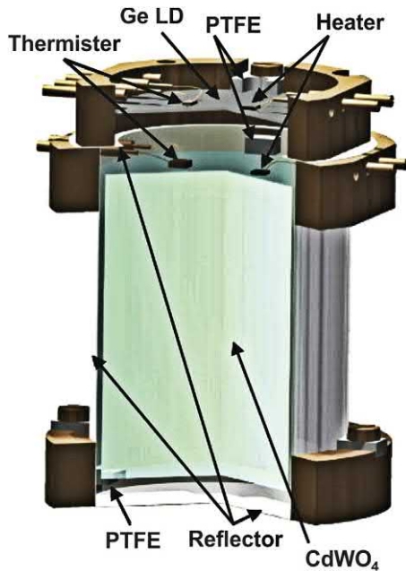
FIGURE 9.124 A single scintillating bolometer with a ^{116}\text{CdWO}_4 crystal. It is held together with four L-shaped Teflon pieces (PTFE) fixed to two cylindrical Cu frames. The frames are held together with two Cu columns (not visible from the chosen perspective). The crystal is surrounded by a 43 mm reflecting sheet. The light detector (Ge LD) consists of a 1 mm thick pure Ge crystal absorber. The surface of the Ge LD facing the crystal is darkened with a 600 Å layer of \text{SiO}_2 to increase light absorption. A resistor of \sim 300 \text{ k}\Omega is attached to each absorber and acts as a heater to stabilize the gain of the bolometer. From Arnaboldi et al. (2010); reprinted with permission from Elsevier © 2010.
