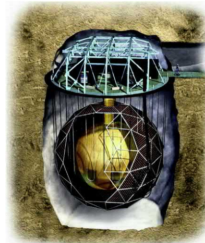
FIGURE 6.111 Cut-away view of the SNO+ detector. The inner 12 m diameter acrylic sphere contains the active volume of Te-loaded liquid scintillation fluor cocktail. A 54% optical coverage is provided by \sim 9500 photomultiplier tubes (PMTs) placed along the inner walls of a 17 m diameter geodesic structure with interior and exterior shielding by pure water. The PMTs are illustrated as bright dots within the triangular panes of the outer structure. For a perspective of the detector dimensions, a person is illustrated walking toward the upper deck in the cave to the right. From Kamdin (2015); reprinted with permission from Elsevier © 2015. For the color version of this figure, the reader is referred to the online version of this book.
