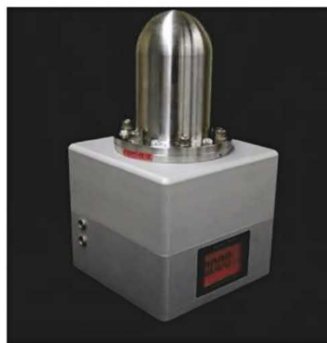
FIGURE 2.32 (A) Schematic drawing and (B) photograph of a tissue-equivalent proportional counter for proton therapy. For the color version of this figure, the reader is referred to the online version of the book. From Nam et al. (2015), reprinted with permission from the Korean Physical Society © 2015.
