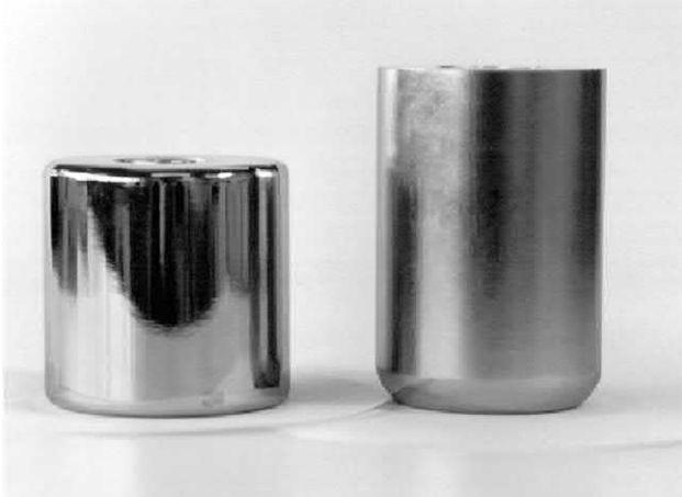
FIGURE 4.22 Two germanium crystals yielding a relative efficiency of 35%. The entrance windows are facing down. The right crystal has rounded edges at the window side.
