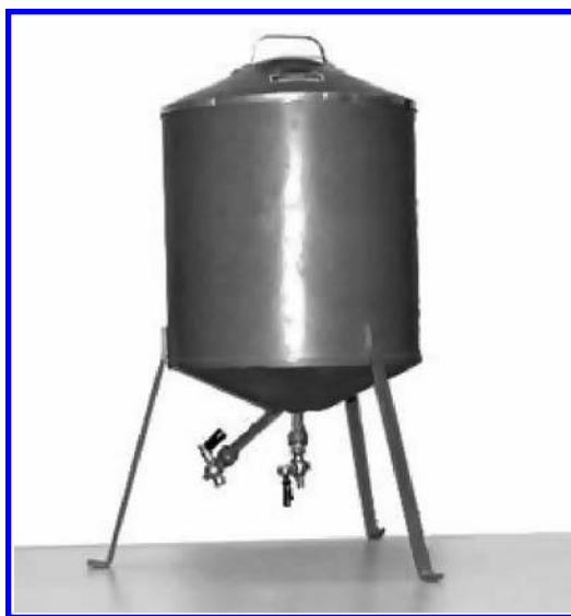
FIGURE 1.6 The ice calorimeter that Lavoisier used to measure the heat given off by a guinea pig calculated from the amount of ice that was melted and the amount of melted ice when a candle was burned to produce heat. When the heat production was similar to the amount of fixed air (carbon dioxide) produced for a guinea pig or a candle, this led to the conclusion that metabolism was like a slow combustion.
