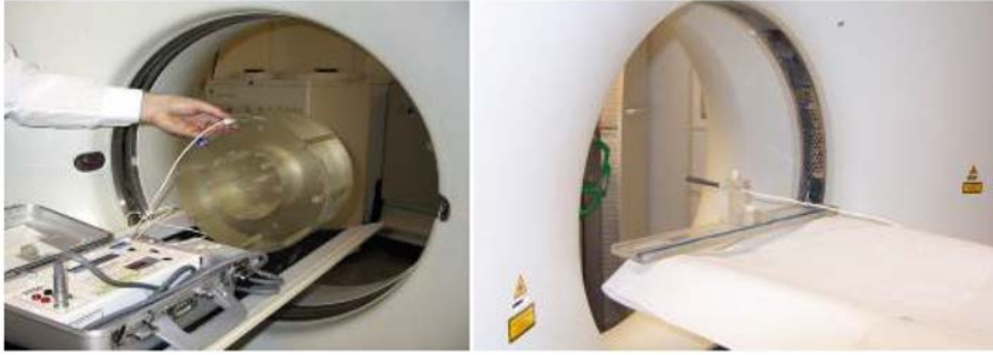
FIG. 23. Measurement of dose in a standard CTDI PMMA body phantom (left) and in air (right).
