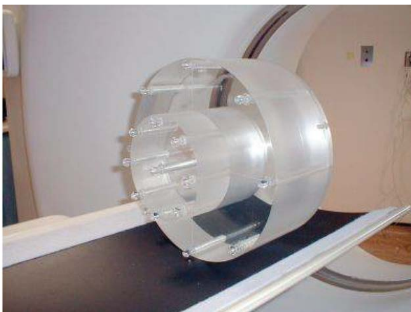
FIG. 37. Photograph of typical standard head and body CT dosimetry phantoms. The head phantom is the innermost cylinder (which has been partially removed for clarity) and when surrounded by a PMMA annulus, the body phantom is formed (from Ref. [26]).
