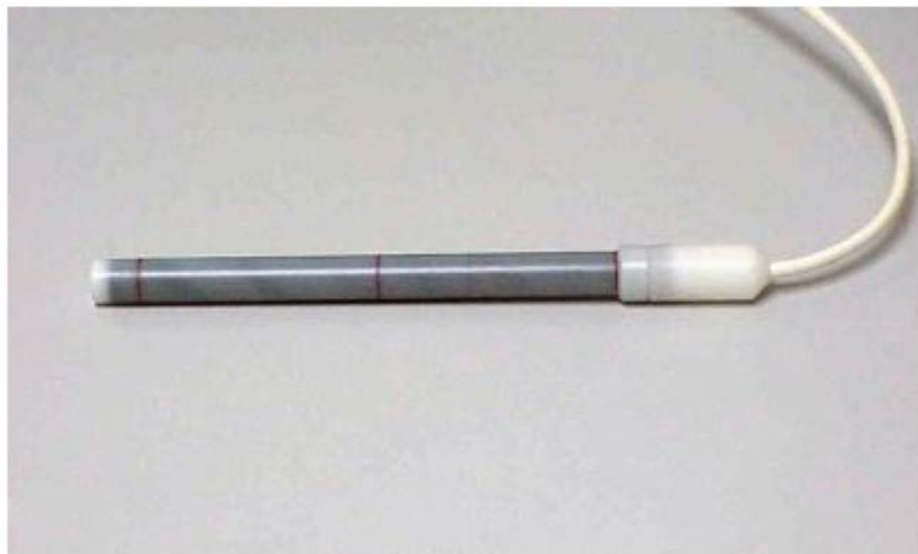
FIG. 39. Pencil ionization chamber used for dosimetry of CT examinations. The active volume of the chamber is typically 3 \text{ cm}^3 and the active length is 100 mm [26].
