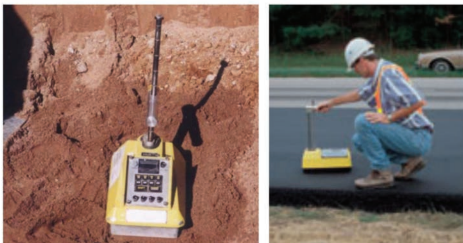
FIGURE 14.4 Moisture density gauges, used in the laying of tarmacadam road surfaces, contain small quantities of both americium-241 and cesium-137. About 22,000 are in use in the United States, and 50 or more are reported lost or missing each year. This material would be suitable to construct a “dirty bomb.”
