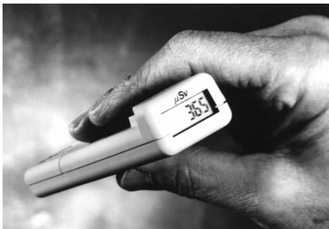
FIGURE 5.6 A personal bleeper radiation monitor. Bleep rates: Background: 1 bleep/15–30 min; 1 mR/h: 1 bleep/20 s; 100 mR/h: continuous alarm signal. (Courtesy of Fluke Biomedical, Cleveland, OH.)
