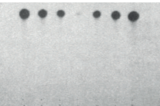
Fig. 13e. Thin-layer chromatogram of iopromide on a silica gel plate 60F-254 (Merck). Solvent: dioxane (85)-water (15)-ammonia (4). Amounts applied from left to right: 200 µg, 100 µg, 50 µg, 1 µg, 50 µg, 100 µg, 200 µg. Photograph taken at 254 nm
