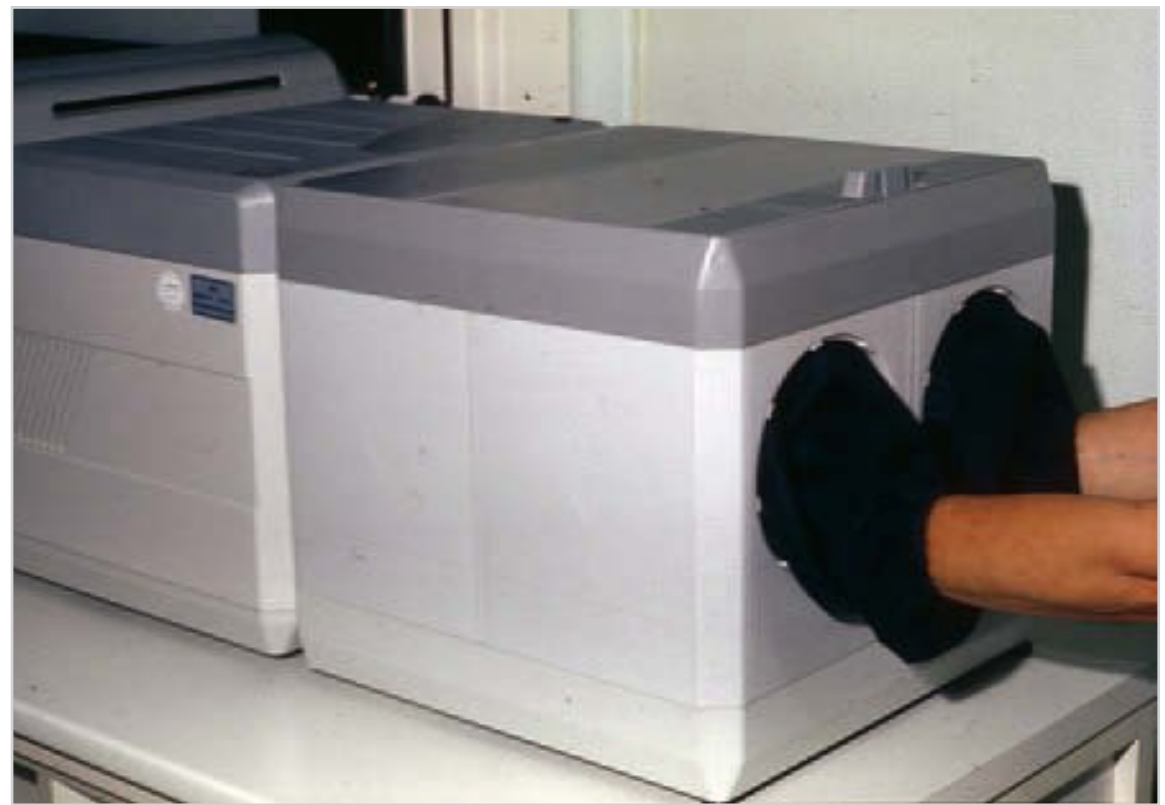
Fig. 6.19 Automatic processor with daylight loading apparatus.
