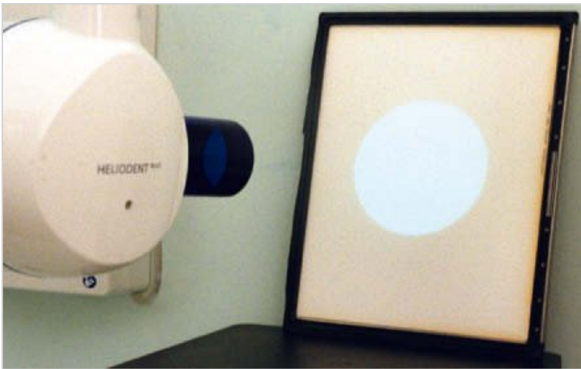
Fig. 2.16 X-ray beam generates light on an intensifying screen.
