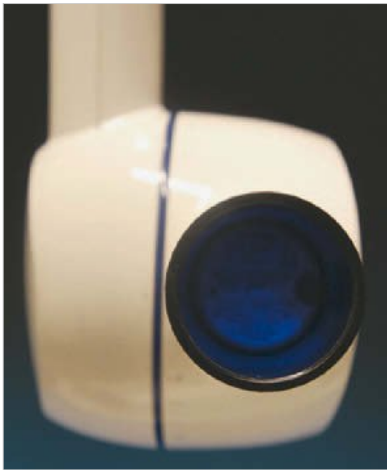
Fig. 2.18 Round cone with a round collimator and a radiation field of 6 cm.
