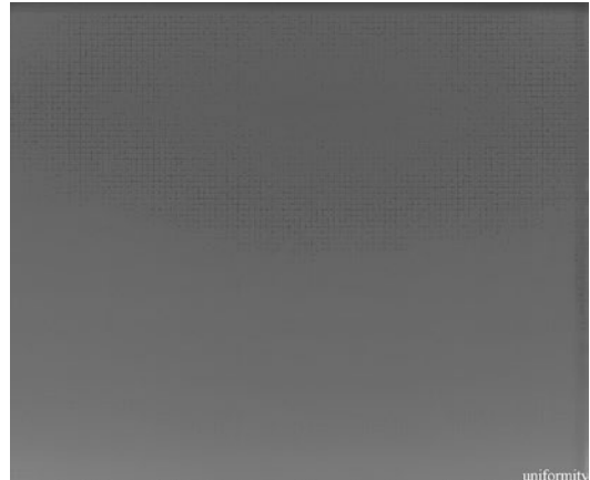
Fig. 11.17 Qualitative criterion for acceptance for the CR IP QC test for uniformity is a uniform image without artifacts
