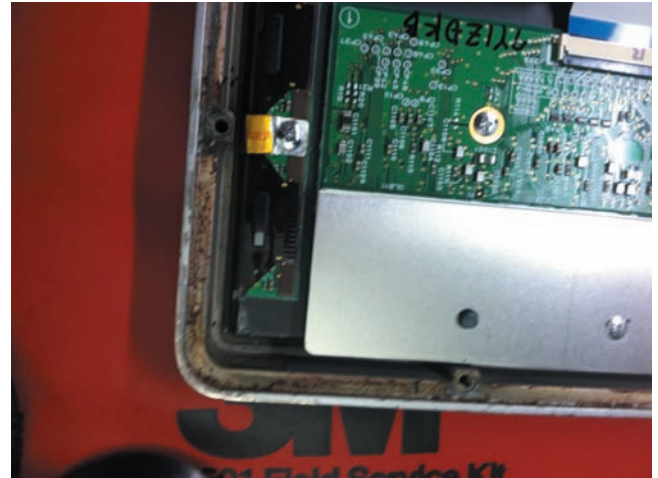
FIGURE 22-8. A damaged DR panel with fluid invasion, due to blood and Betadine.
