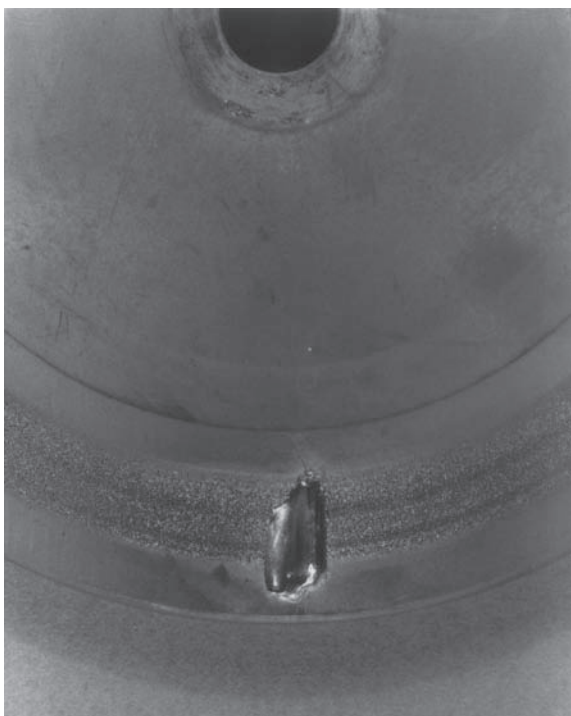
FIGURE 5-19. Anode melt due to rotor-bearing failure.
