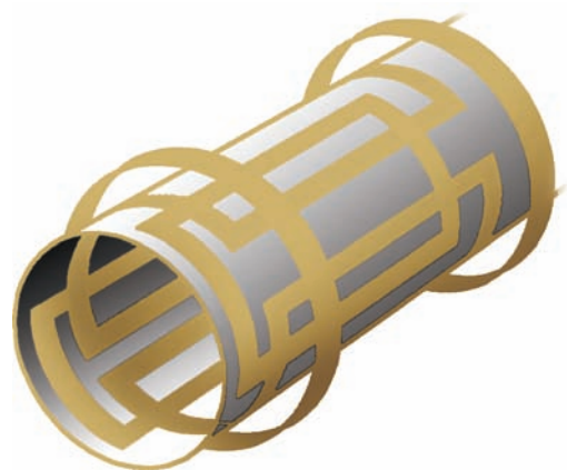
FIGURE 39-5. Gradient coil windings within the magnetic enclosure.
