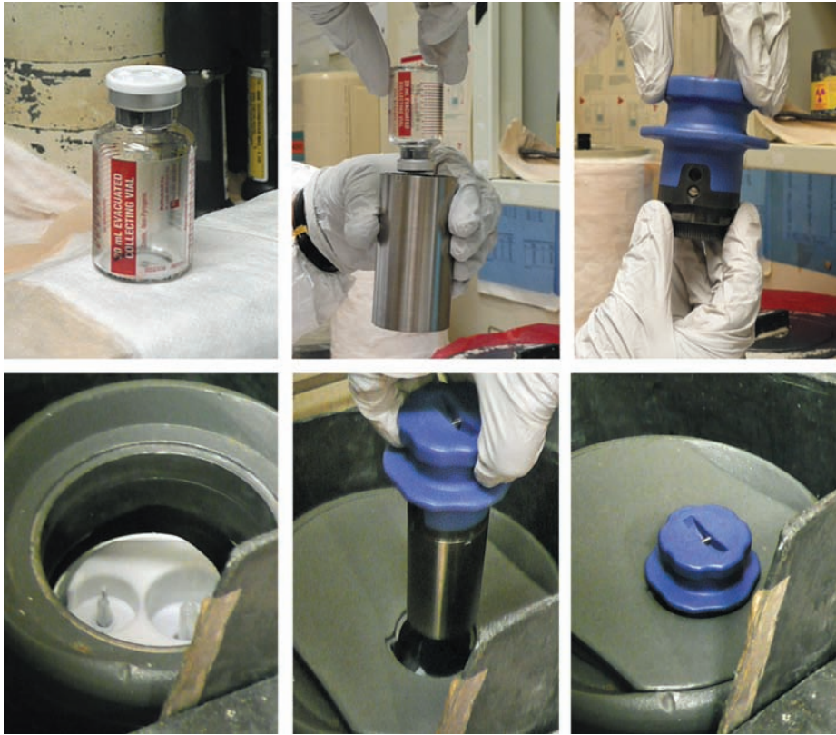
FIGURE 40-6. Eluting the radionuclide generator. The evacuated vial is placed inside a specially designed shield that fits onto the elution needle projecting from the top of the generator. After a few minutes, the vial can be removed and will contain the generator eluate ready for quality control testing and patient use.
