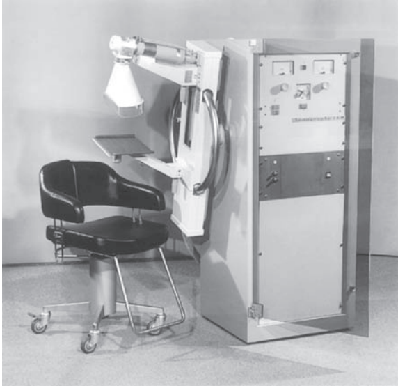
FIGURE 35-1. A 1967 Senograph, produced by CGR (France), became the first commercially available dedicated mammography machine. The unit contained the first molybdenum anode, 0.7-mm focal spot, beryllium window port, and compression device.
