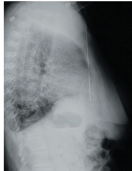
FIGURE 22-6. Note the white line, which is caused by a column of bad detector elements in the TFT. This requires a system calibration, and then can be used again.
