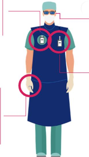
The **dosimeter placed at the eyes level** provides an estimation the **dose to the eye lens**.
