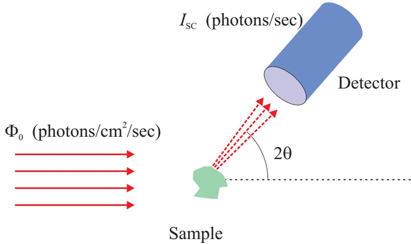
**Fig. 5.17** Scattering from a small crystal. The incident beam is assumed to be perfectly collimated and monochromatic, and to fully illuminate the crystal. The scattered intensity  $I_{sc}$  is proportional to the flux  $\Phi_0$  and to the differential cross-section ( $d\sigma/d\Omega$ ) of the sample.
