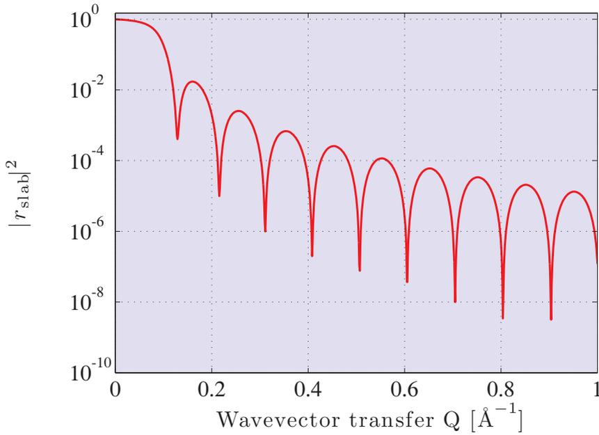
**Fig. 3.7** ★ Kiessig fringes from a homogeneous slab of Tungsten. Solid curve: the calculated reflectivity  $|r_{\text{slab}}|^2$  for a slab of thickness  $10 \times 2\pi \text{ \AA}$ . The density of the film is 4.678 electrons per  $\text{\AA}^3$ , Table 3.1.
