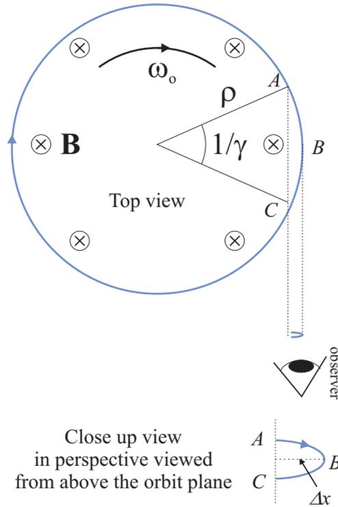
**Fig. 2.4** An electron is kept in a circular orbit by the magnetic field  $\mathbf{B}$ . An observer in the direction of the tangent at point  $B$  will, due to the Doppler effect, see the electron as having a large acceleration when it is between points  $A$  and  $C$ . The close-up view indicates that the observer will experience something that resembles half a period of an oscillation.
