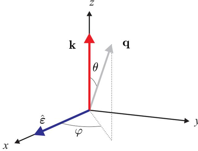
**Fig. 7.3** The coordinate system relating the angles  $(\theta, \varphi)$  to the wavevector of the photoelectron  $\mathbf{q}$  and the wavevector and polarization of the incident photon  $(\mathbf{k}, \hat{\boldsymbol{\epsilon}})$ . In this case the photon propagates along the  $z$  direction and has its electric field polarized along  $x$ .
