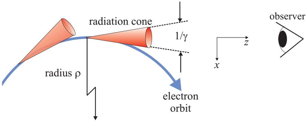
**Fig. 2.2** A relativistic electron moving in a circular trajectory of radius  $\rho$ . The radiation emitted is confined to a narrow cone with an opening angle of  $1/\gamma$  around the instantaneous velocity.
