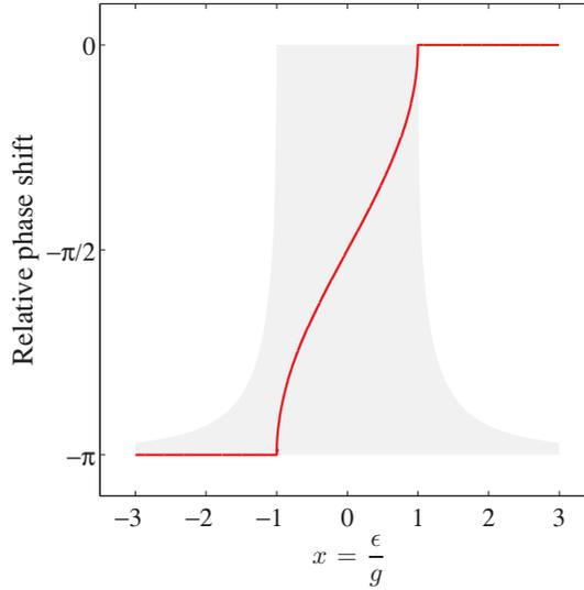
**Fig. 6.6** The relative phase shift between the incident  $T_0$  and reflected  $S_0$  wavefields as calculated from Eq. (6.20). For reference, the Darwin curve is shown in shaded relief in the background. The two wavefields are out of phase, here chosen to be  $-\pi$ , for  $x \leq -1$ , and in phase for  $x \geq 1$ .
