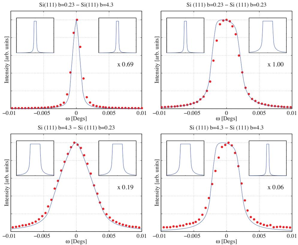
**Fig. 6.12** Measured rocking curves for a double crystal diffractometer formed from two asymmetric perfect silicon crystals. The solid lines represent the calculated convolution of two Darwin curves with widths determined by how the asymmetric crystals were configured.
