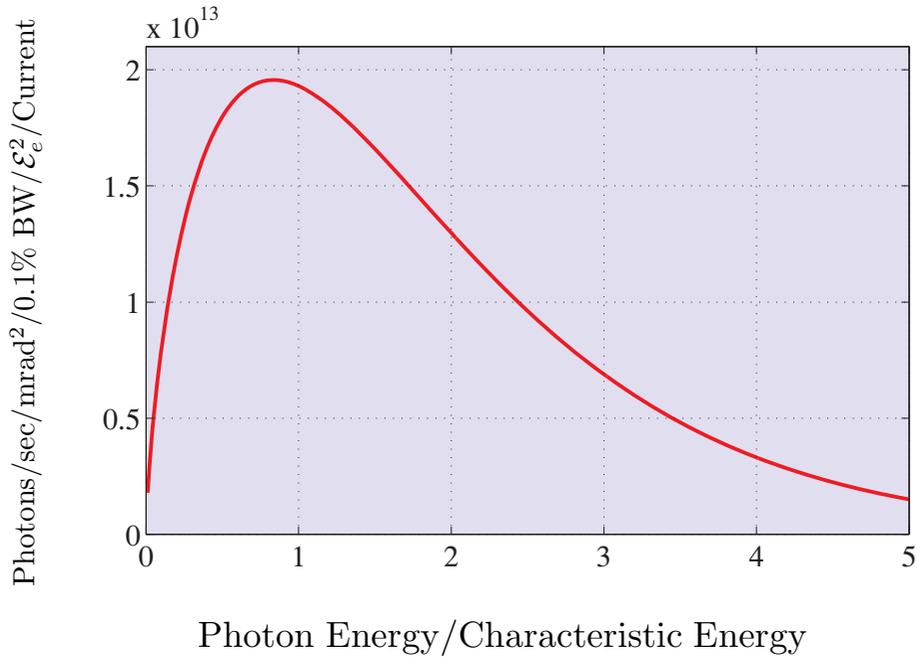
**Fig. 2.6** The spectrum from a bending magnet, normalised by the square of the electron energy and the beam current. The abscissa is  $x = \hbar\omega/(\hbar\omega_c)$ , i.e. the photon energy normalized by the characteristic energy  $\hbar\omega_c = (\frac{3}{2})\gamma^3\hbar\omega_0$ . The numerical formula is  $1.33 \times 10^{13} x^2 K_{2/3}^2(x/2)$ , where  $K_{2/3}(x/2)$  is a modified Bessel function. The electron energy  $\mathcal{E}_e$  is in GeV, and the beam current in Amperes.
