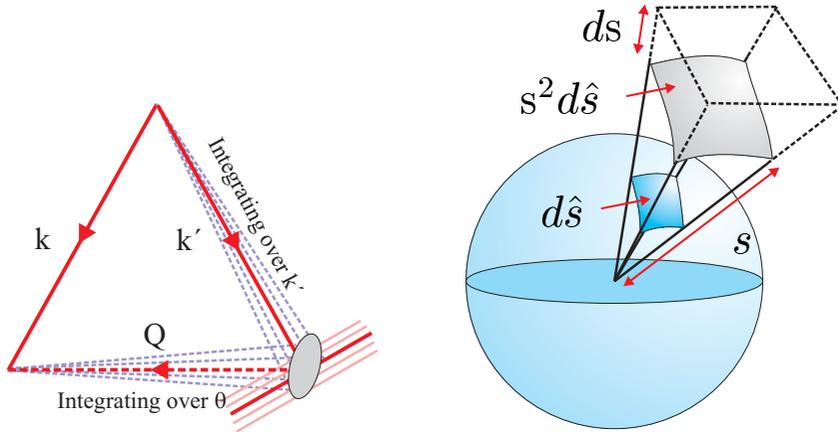
**Fig. 5.18** Left: The scattering from a small crystallite is represented by the grey ellipse, which reflects the reciprocal of the shape of the crystal. For a given orientation of the crystal the detector accepts all of the scattered wavevectors  $\mathbf{k}'$  which fall on the red line. As the crystal is rotated the integration corresponds to the other light red lines. Right: The solid angle element  $d\hat{s}$  and the volume element  $ds$  are related by  $ds = s^2 d\hat{s} ds$ .
