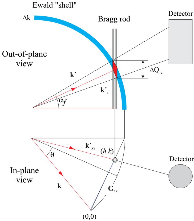
**Fig. 5.22** Reciprocal space diagram for a 2D system showing the intersection of part of the Ewald sphere with the Bragg rod. The in-plane projection of reciprocal space is shown in the bottom part, and the out-of-plane projection in the top.
