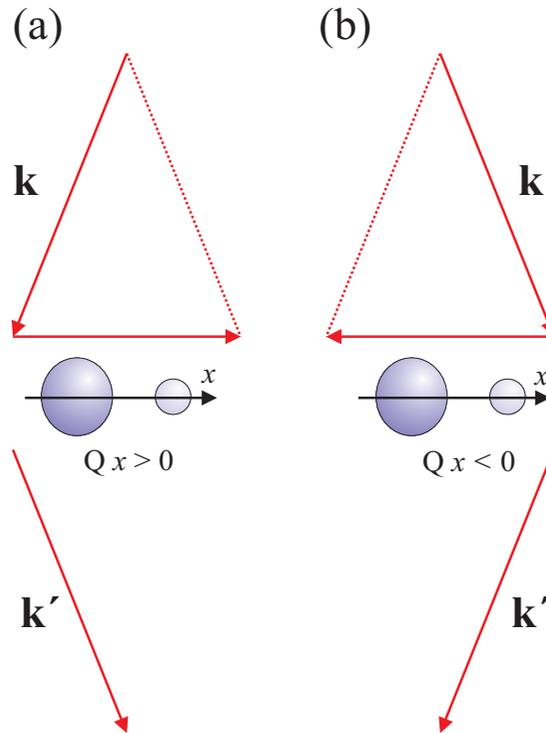
**Fig. 8.6** Diffraction by two non-identical atoms. Analysis of the scattered intensities when the scattering vector is parallel to the direction connecting the large and small atoms, or when it is in the opposite direction, shows that with the dispersion corrections taken into account it is possible to tell whether the large atom is to the right or left of the smaller one.
