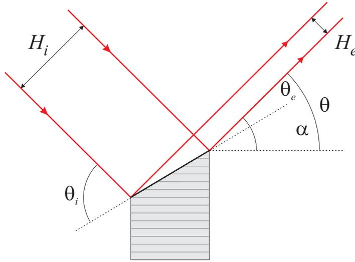
**Fig. 6.11** Asymmetric Bragg reflection. The surface of the crystal is at an angle  $\alpha$  with respect to the reflecting atomic planes. The widths of the incident and scattered beams are then different. In this case the parameter  $b$  is greater than one.
