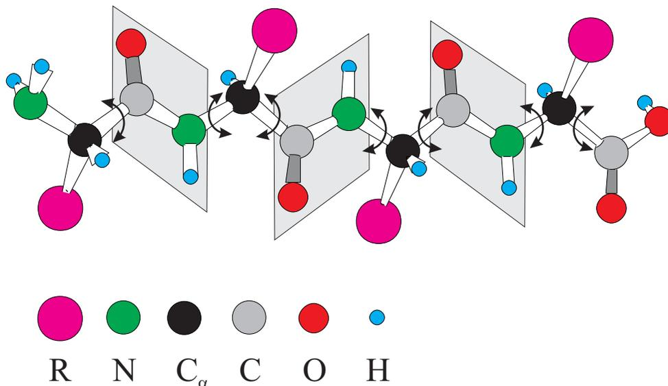
**Fig. 5.26** A polypeptide chain is composed of planar moieties of carbonyl and amide groups. These planar moieties can be rotated around either the  $N-C_\alpha$  or the  $C_\alpha-C$  bonds. Hydrogen bonding between the  $N-H$  and  $C=O$  groups causes the chain to fold into a helical structure known as the  $\alpha$ -helix after Pauling. Here  $R$  stands for an amino acid residue.
