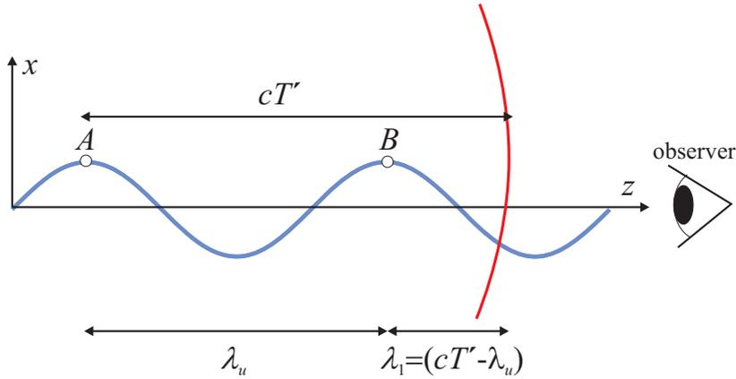
**Fig. 2.8** Constructive interference occurs when the wavefront emitted by the electron when it was at  $A$  is one wavelength  $\lambda_1$  ahead of the wavefront emitted by the electron when it reaches  $B$ . This is then the fundamental wavelength emitted from the undulator.
