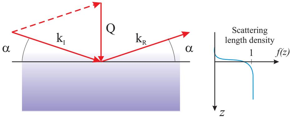
**Fig. 3.10** A flat interface with a graded density given by the shape function  $f(z)$ , normalized to unity at large  $z$ . The Fourier transform of its derivative,  $\phi(Q)$ , can be considered to be the form factor of the density variation across the interface.
