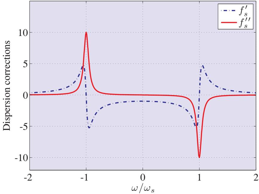
**Fig. 8.2** The real,  $f'_s$ , and imaginary,  $f''_s$ , parts of the dispersion corrections as a function of the driving frequency  $\omega$  relative to the resonant frequency  $\omega_s$  calculated for a single oscillator model. In the example shown here the damping  $\Gamma$  has been chosen to be equal to  $0.1 \omega_s$ .
