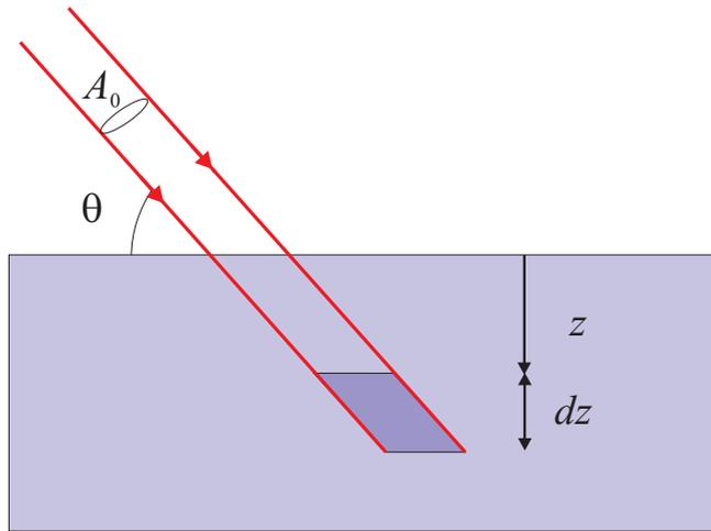
**Fig. 5.20** Extended face geometry. A beam of X-rays is incident on the flat face of a crystal at an angle  $\theta$ . The cross-sectional area of the beam is  $A_0$ , and the illuminated volume of sample at a depth of  $z$  from the surface is  $(A_0/\sin\theta)dz$ .
