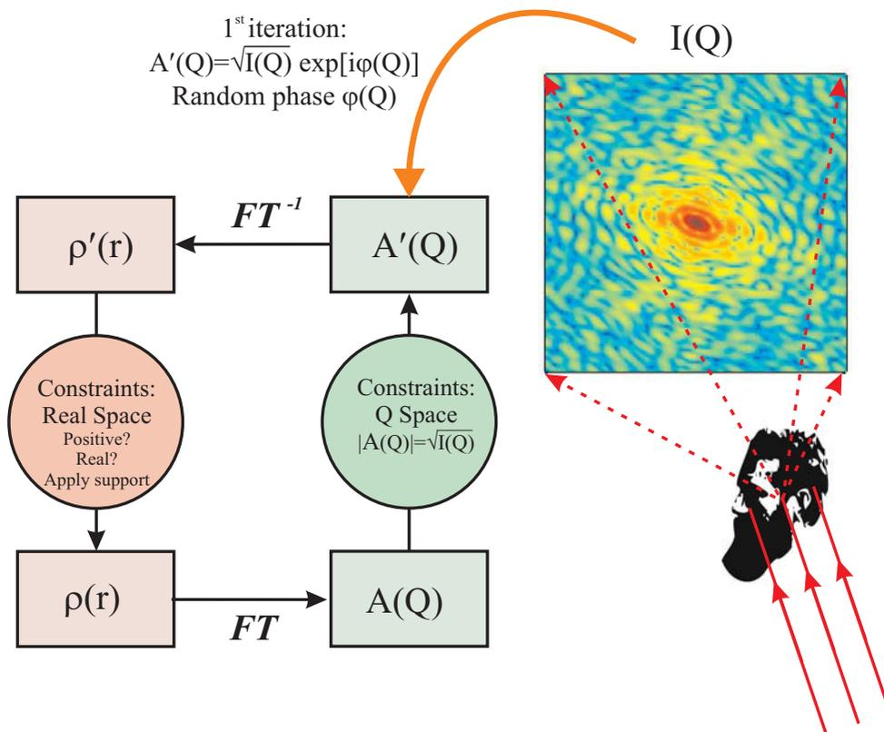
**Fig. 9.21** Schematic of the iterative, phase retrieval algorithm used to reconstruct real space images from coherent X-ray diffraction images. In the right hand panel a test object is illuminated by a coherent X-ray beam and the diffracted intensity,  $I(Q)$ , is recorded on a position sensitive area detector placed in the far-field. The diffraction pattern in this case is that of a portrait of W.C. Röntgen.
