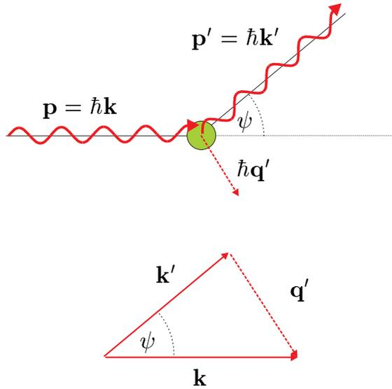
**Fig. 1.9** Compton scattering. A photon with energy  $\mathcal{E} = \hbar ck$  and momentum  $\hbar\mathbf{k}$  scatters from an electron at rest with energy  $mc^2$ . The electron recoils with a momentum  $\hbar\mathbf{q}' = \hbar(\mathbf{k} - \mathbf{k}')$  as indicated in the scattering triangle in the bottom half of the figure.
