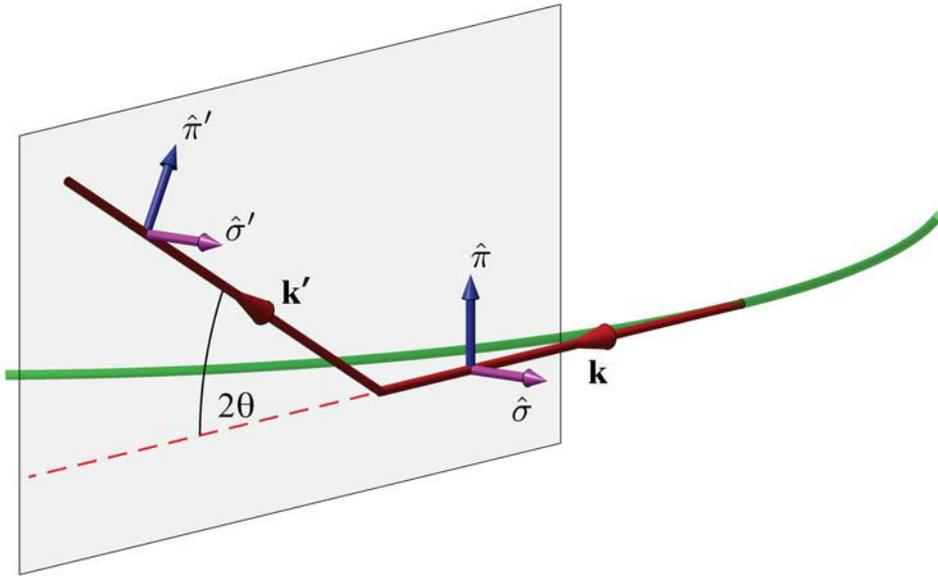
**Fig. 2.5** Illustration of the vertical scattering geometry typically employed at synchrotrons. The component of the X-ray's electric field perpendicular to the scattering plane is labelled  $\hat{\sigma}'$ , while the component in the plane is labelled  $\hat{\pi}$ . When viewed exactly in the orbit plane the radiation from an electron traversing a circular arc is purely  $\hat{\sigma}'$  polarized.
