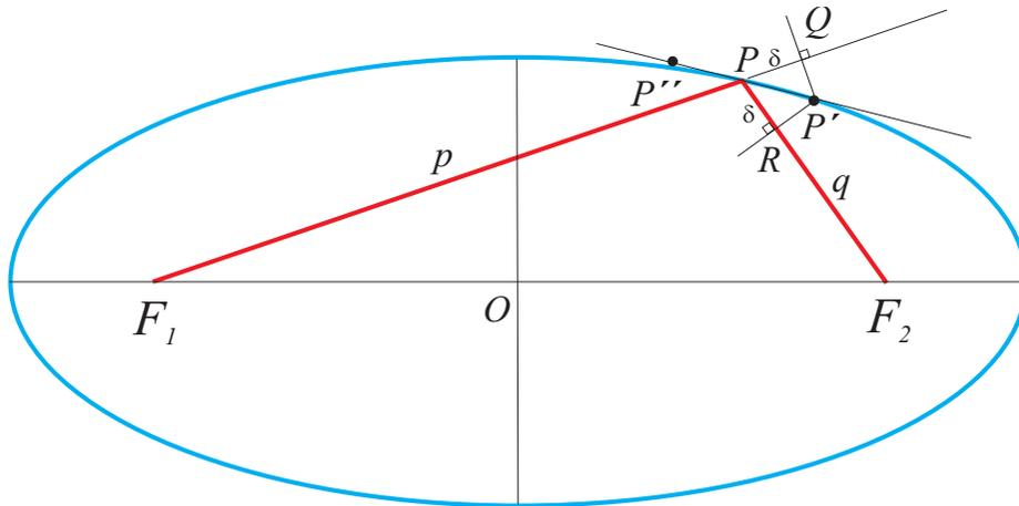
**Fig. 3.19** Elementary proof that the tangent in a point of an ellipse bisects the angle of the rays from the two foci to the point. The angle  $RPP'$  is equal to the angle  $QPP'$  and hence a ray from  $F_1$  will be focused at  $F_2$ .
