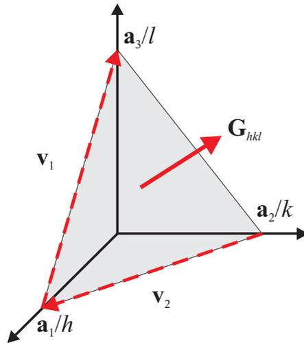
**Fig. 5.4** (a) The equivalence of Bragg's Law and the Laue condition for the particular case of the 2D square lattice. (b) Construction to prove that the reciprocal lattice vector  $\mathbf{G}_{hkl}$  is perpendicular to the  $(h, k, l)$  planes, and has a magnitude equal to  $2\pi/d_{hkl}$ .
