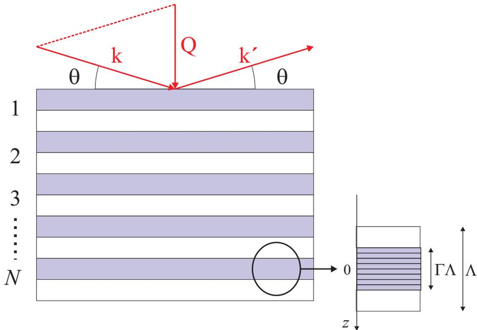
**Fig. 3.8** Schematic of a multilayer which here is a stack of bilayers. Each bilayer, as shown to the right has a homogeneous high electron density region of thickness  $\Gamma\Lambda$ , and a low density region. The total thickness of a bilayer is  $\Lambda$ .
