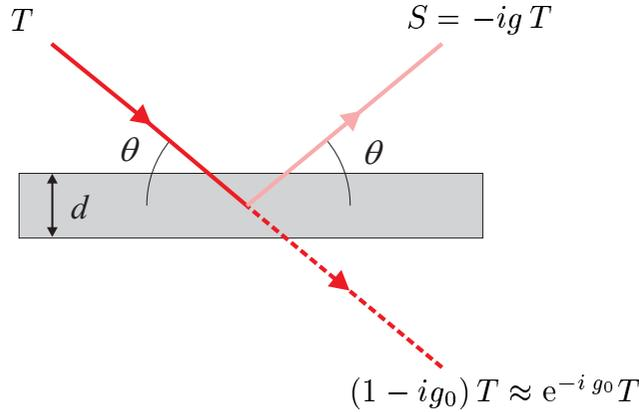
**Fig. 6.2** A wave  $T$  incident on a sheet of unit cells will be partly reflected and partly transmitted. The reflected wave is  $-igT$ , and the transmitted wave is  $T(1 - ig_0)$ , where  $g$  and  $g_0$  are small parameters given in the text.
