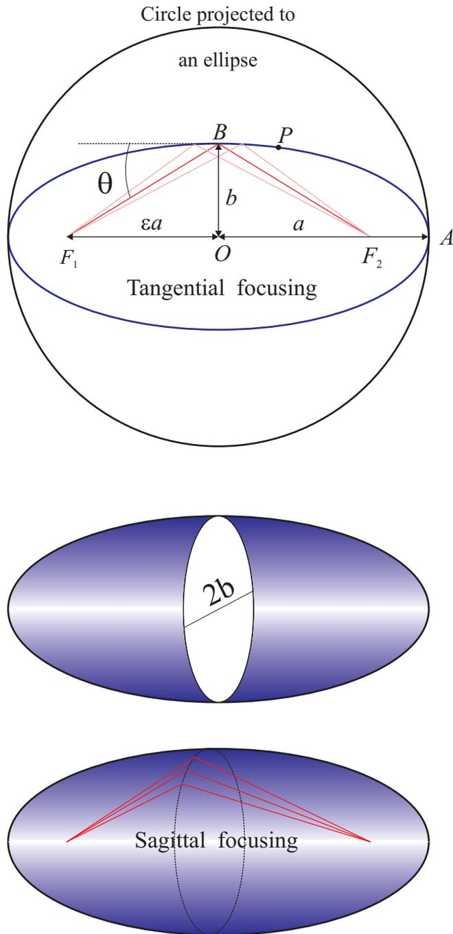
**Fig. 3.20** By considering an ellipse as a projection of a circle (top), which is the same as a contraction of the vertical axis by the factor  $(b/a)$ , one realizes that the radius of curvature at  $B$  must be the radius of the circle,  $a$ , divided by  $(b/a)$ . Considering the ellipsoid (middle and bottom) it is clear that the best sagittal radius at  $B$  must be  $b$ .
