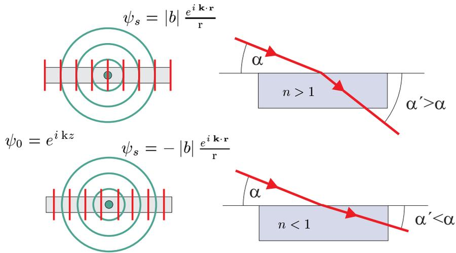
**Fig. 3.1** The spherical wave  $\psi_s$  from a point scatterer can be in phase (top) or  $180^\circ$  out of phase with the incident plane wave  $\psi_0$  (bottom). The refractive index is greater than unity in the first case, and smaller than unity in the second case.
