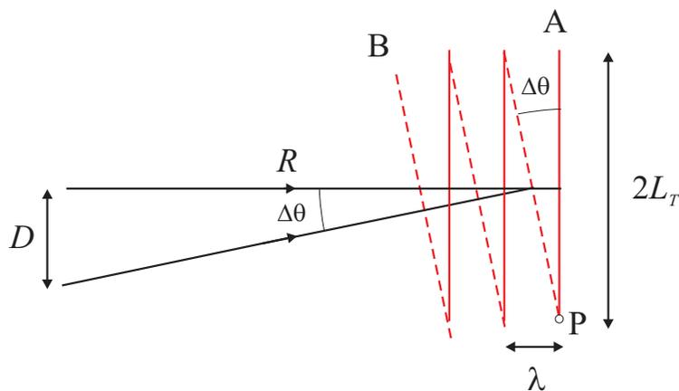
**Fig. 1.16** Longitudinal and transverse coherence lengths. (a) Two plane waves with different wavelengths are emitted in the same direction. For clarity we have shown the waves displaced from each other in the vertical direction. After a distance  $L_L$ , the longitudinal coherence length, the two are out of phase by a factor of  $\pi$ . (b) Two waves with the same wavelength are emitted from the ends of a finite sized source of height  $D$ .
