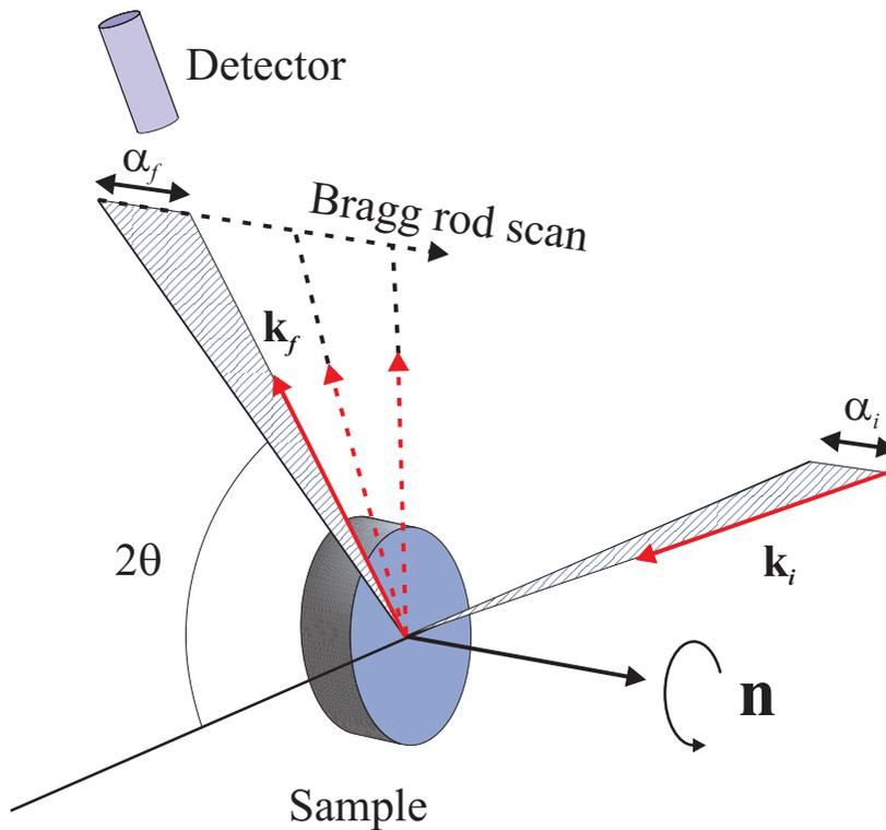
**Fig. 5.29** Geometry of a grazing incidence diffraction (GID) experiment from a solid single crystal surface at a synchrotron. The surface can be rotated around the surface normal  $\mathbf{n}$ , and the detector can be both rotated around  $\mathbf{n}$  in the vertical plane, and moved perpendicular to it so as to scan along the crystal truncation rods.
