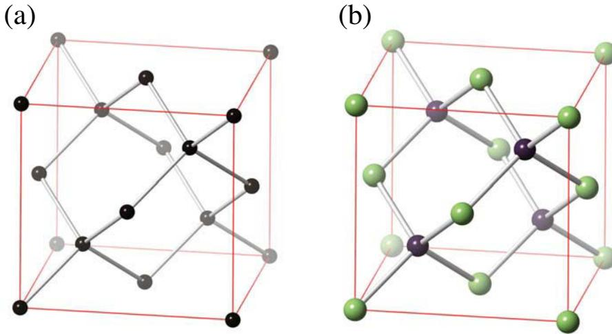
**Fig. 5.5** The diamond lattice (a) can be formed from two inter-penetrating *fcc* lattices displaced by  $(\frac{1}{4}, \frac{1}{4}, \frac{1}{4})$  with respect to each other. For the zinc sulfide (also known as zinc blende) structure (b) the two lattices are occupied by different types of atom.
