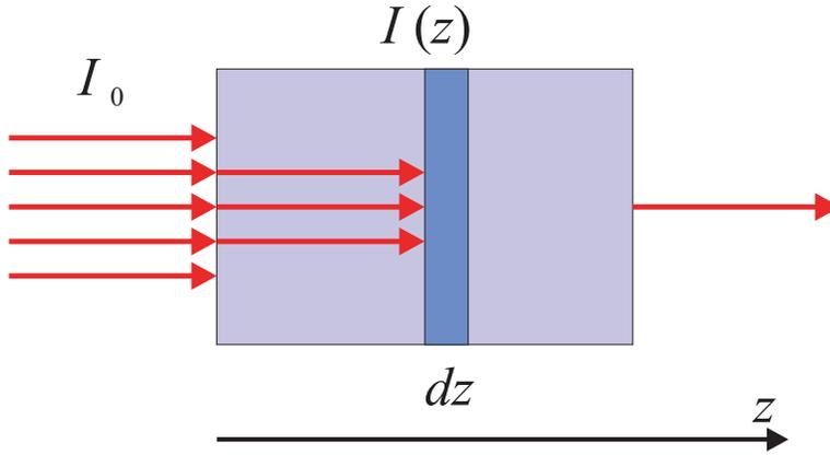
**Fig. 1.12** The attenuation of an X-ray beam through a sample due to absorption. The attenuation follows an exponential decay with a characteristic linear attenuation length  $1/\mu$ , where  $\mu$  is the absorption coefficient.
