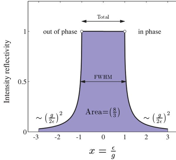
**Fig. 6.5** The Darwin reflectivity curve calculated from Eq. (6.21). For values of  $x$  between  $-1$  and  $1$  the reflectivity is 100%. This is known as the region of total reflection. For large values of  $|x|$  the intensity decays as  $1/(2x)^2$ . At  $x = 1$  the X-ray wavefield has its maxima on the atomic planes, whereas for  $x = -1$  the nodes of the wavefield coincide with the atomic planes.
