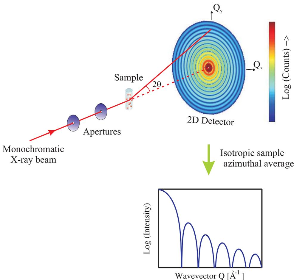
**Fig. 4.11** Schematic layout of a small-angle X-ray scattering beamline. A monochromatic X-ray beam is collimated using a set of apertures and then impinges on the sample. The scattered beam is detected on a two-dimensional, position sensitive detector (PSD). For isotropic samples, the scattering can be azimuthally averaged to produce a plot of scattered intensity versus wavevector transfer.
