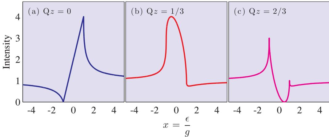
**Fig. 6.8** Illustration of the sensitivity of the intensity of X-ray standing waves to  $Qz$ . The solid lines have been calculated from Eq. (6.37) using the phase  $\phi$  and the modulus of the amplitude reflectivity  $|r|$  obtained from Eq. (6.20).
