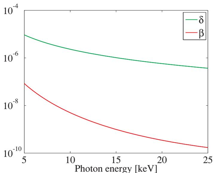
**Fig. 9.10** The energy dependence of the real ( $\delta$ ) and imaginary ( $\beta$ ) contributions to the refractive index of water. Although it might be expected that  $\beta$  of water is low – due to the weakness of the absorption cross-section – it turns out that in the hard part of the X-ray spectrum, above 5 keV or so,  $\delta$  exceeds  $\beta$  in all materials.
