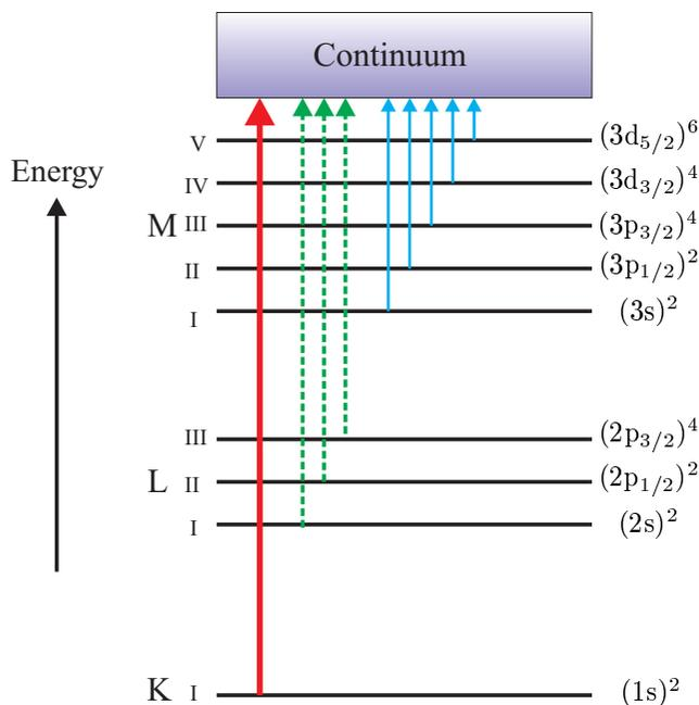
**Fig. 7.2** A summary of the nomenclature used to label the absorption edges of the elements. The K edge corresponds to the energy required to remove an electron from the 1s shell to the continuum of free states, etc. The electronic shells are labelled as  $(n\ell_j)^{2j+1}$ , where  $n$ ,  $\ell$  and  $j$  are the principal, orbital angular momentum, and total angular momentum quantum numbers, respectively, of the single-electron states. The multiplicity is  $2j + 1$ .
