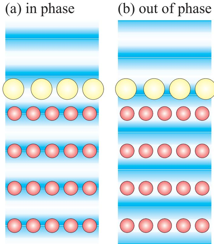
**Fig. 6.7** The standing wavefield changes phase with respect to the lattice planes throughout the region of total reflectivity. (a) On one side ( $x = 1$ , Fig. 6.5) the standing wave has nodes between the lattice planes, and on the other side (b) ( $x = -1$ ) at the lattice planes. The standing wavefield extends beyond the crystal surface, and the height of an absorbed layer (represented by larger circles) can be determined by their fluorescent yield vs the phase of the standing wave.
