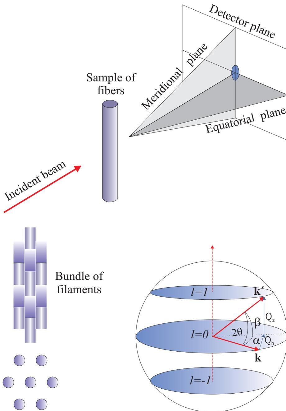
**Fig. 5.25** Top: geometry of fibre diffraction. The fibre sample is perpendicular to the incident monochromatic beam. Bottom left: the fibre sample comprises a large number of filaments, randomly orientated in the azimuthal angle. Bottom right: periodicity along the fibre implies that Bragg reflections are restricted to layers.
