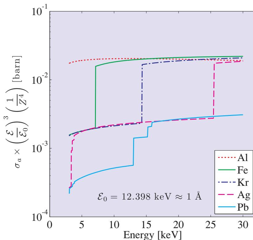
**Fig. 7.1** The scaled absorption cross-section as a function of photon energy for a selection of elements. The absorption cross-section per atom,  $\sigma_a$ , has been scaled by dividing it by the atomic number  $Z$  to the fourth power, and multiplying it by the photon energy  $\mathcal{E}$  to the third power.
