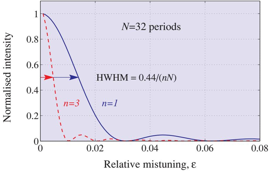
**Fig. 2.12** Monochromaticity of the first ( $n = 1$ ) and third ( $n = 3$ ) harmonic for an undulator with  $N = 32$  periods as seen through an on-axis pin hole from a zero emittance source. The monochromaticity half width at half maximum (HWHM) is approximately equal to  $0.44/(nN)$ .
