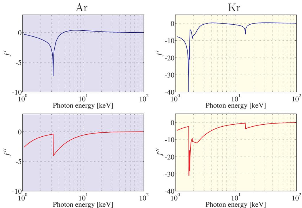
**Fig. 8.5** The calculated energy dependence of the real,  $f'$ , and imaginary,  $f''$ , parts of the dispersion corrections (in units of  $r_0$ ) for Ar and Kr. The calculations were performed within the self-consistent Dirac-Hartree-Fock framework, and are discussed in the text. The K edge of Ar is evident at 3.203 keV. For Kr the K edge occurs at 14.32 keV, while the L edges are centred around 1.8 keV.
