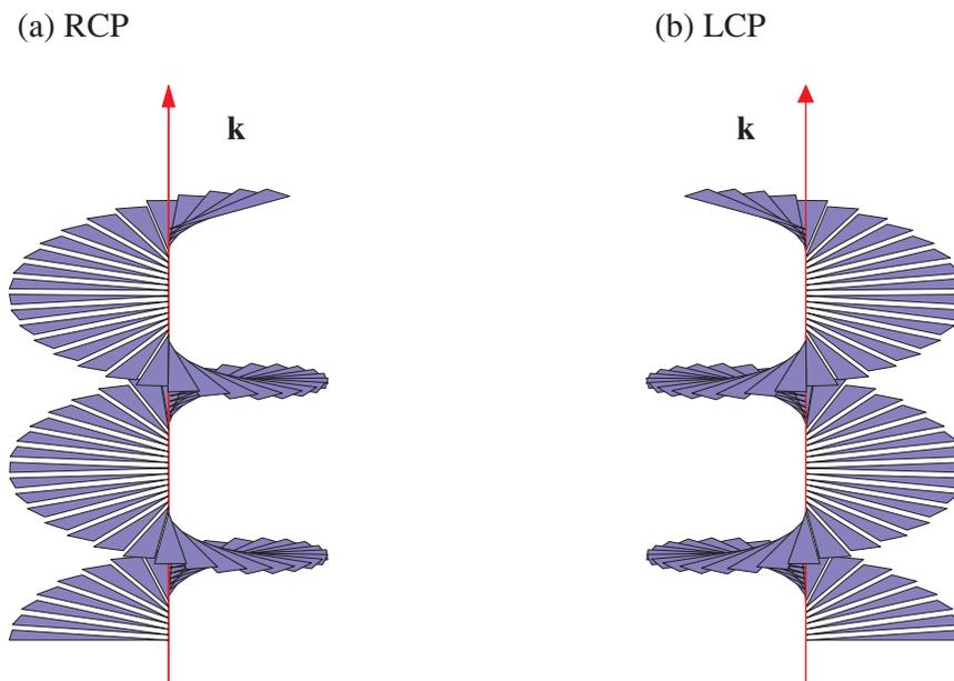
**Fig. 7.11** Circular polarized X-rays can be depicted as a helical staircase where the steps in the staircase represent the electric field vector. The two possible polarization states correspond to the staircase turning clockwise along the direction of propagation  $\mathbf{k}$  (right circularly polarized, RCP), or anticlockwise (left circularly polarized, LCP).
