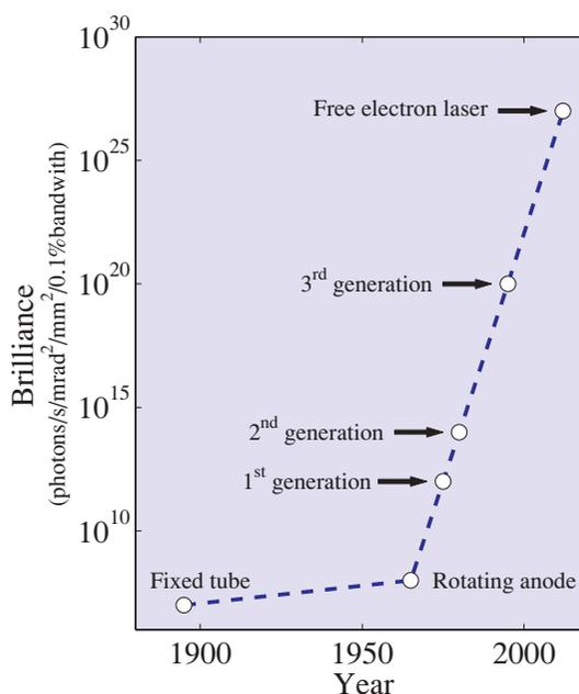
**Fig. 1.1** The brilliance of X-ray sources as a function of time. Source brilliance is defined and discussed in Chapter 2, along with the principles underlying the production of X-rays from synchrotrons and free-electron lasers. For free-electron laser sources we plot the average brilliance. Due to the extremely short X-ray pulse length from a free-electron laser – of order 100 fs – the peak brilliance exceeds the average brilliance by a large factor.
