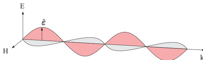
**Fig. 1.4** An X-ray is a transverse electromagnetic wave, where the electric and magnetic fields,  $\mathbf{E}$  and  $\mathbf{H}$ , are perpendicular to each other and to the direction of propagation  $\mathbf{k}$ . The direction of the electric field is given by the polarization unit vector  $\hat{\mathbf{e}}$ .
