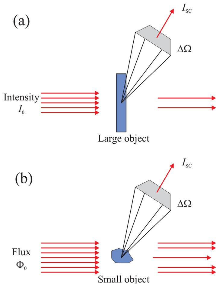
**Fig. A.1** (a) A beam is incident on a sample with a larger cross-sectional area. In this case the intensity  $I_{sc}$  scattered into a solid angle  $\Delta\Omega$  is proportional to the incident *intensity*  $I_0$  of the beam, i.e. the number of photons per second. (b) A beam is incident on a sample with a smaller cross-sectional area. Now the scattered intensity  $I_{sc}$  is proportional to the incident *flux*  $\Phi_0$  of the beam, i.e. the number of photons per second per unit area.
