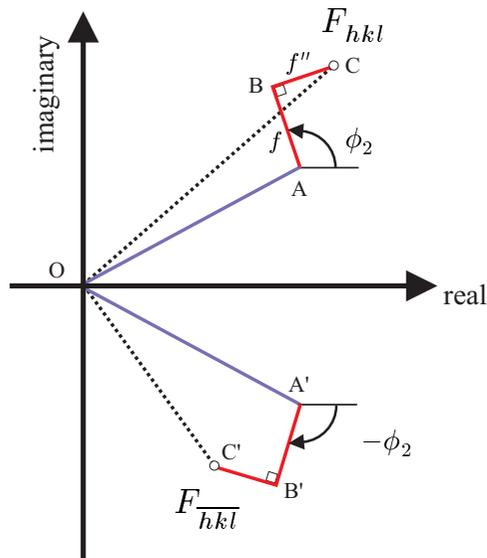
**Fig. 8.7** Argand diagram for a unit cell structure factor. (a) One atom per unit cell neglecting dispersion corrections. In this case  $|F_{hkl}| = |F_{\bar{h}\bar{k}\bar{l}}|$ . (b) Adding one more atom, with dispersion corrections, to the unit cell will change the structure factors to be  $F_{hkl} = OC$  and  $F_{\bar{h}\bar{k}\bar{l}} = OC'$ . In this case  $|F_{hkl}| \neq |F_{\bar{h}\bar{k}\bar{l}}|$ .
