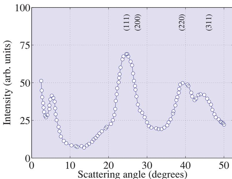
**Fig. 7.8** Powder diffraction data for CdTe nano-crystals with an average diameter of around 15 Å. The X-ray wavelength was 1.54 Å. The graph was prepared by digitising the data of Rogach et al. [1996]
