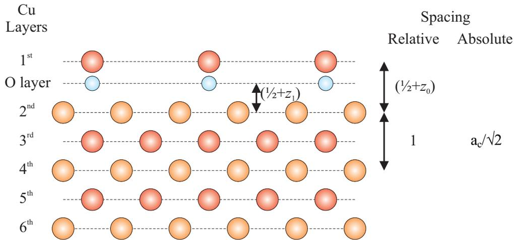
**Fig. 5.32** Schematic of the side view of O on Cu(110) surface showing the possible displacements perpendicular to the surface of the oxygen and copper atoms  $z_1$  and  $z_0$  respectively. The view is along the  $\mathbf{b}$  axis of Fig. 5.30, and the displacements are not to scale.
