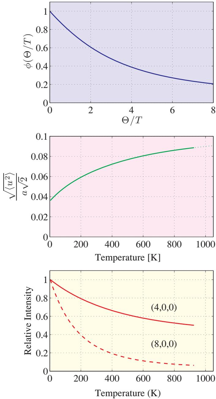
**Fig. 5.16** ★ Top: plot of the value of the integral  $\phi(x)$  versus  $x = \Theta/T$ . Middle: temperature dependence of the rms fluctuation  $\mathbf{u}$  in units of  $a/\sqrt{2}$  for Al. Bottom: the relative intensity of the scattered intensity from Al as a function of temperature. The curves were calculated for the (4,0,0) (solid line) and the (8,0,0) (dashed line) Bragg peaks respectively. The melting temperature of Al is 933 K.
