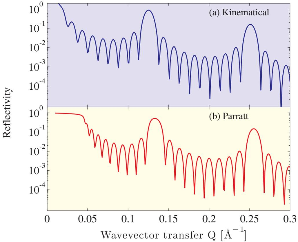
**Fig. 3.9** ★ Specular reflectivity from a W/Si multilayer: 10 bilayers each being 10 Å (amorphous) W on 40 Å (amorphous) Si. (a) Kinematical reflectivity. (b) Reflectivity curve calculated using Parratt's method. The parameters used in the calculation were taken from Table 3.1.
