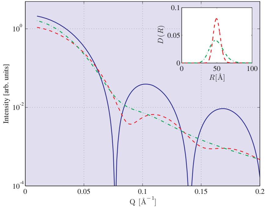
**Fig. 4.15** ★ Effect of polydispersity on the calculated SAXS curve. Solid blue line: form factor of a spherical particle, radius  $R=50 \text{ \AA}$  (Eq. (4.23)). Dashed red line: average form factor for particles described by a Schulz distribution (Eq. (4.29)) with  $\bar{R}=50 \text{ \AA}$  and a polydispersity of  $p=10 \%$  ( $z=99$ ) (see inset). Dot-dashed green line: average form factor for particles described by  $\bar{R}=50 \text{ \AA}$  and  $p=20 \%$  ( $z=24$ ) (see inset).
