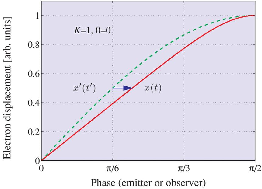
**Fig. 2.10** Construction to show the relationship between the displacement as a function of emitter time for the electron (dashed sinusoidal line) and observer time (solid line). For example, the difference between the emitter,  $\omega_u t'$ , and observer,  $\omega_1 t$ , phases at the point  $\omega_u t' = \pi/6$  is represented by the arrow (see Eq. (2.18)).
