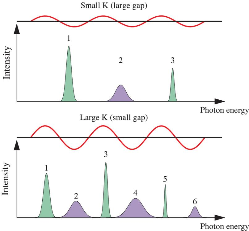
**Fig. 2.14** Schematic of the spectrum from an undulator. The energy of the harmonics can be tuned by  $K$  so that a larger gap, implying a lower field and thereby a smaller  $K$ , gives a higher energy.
