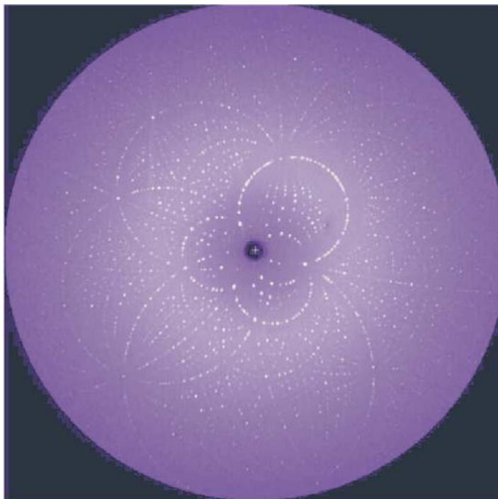
**Fig. 5.8** Pulsed Laue diffraction pattern from the photo-active yellow protein. The diffraction pattern was collected by averaging over 10 exposures, each of 100 ps duration. This image contains about 3700 usable reflections from which the structure could be obtained. (Data courtesy of Michael Wulff, European Radiation Facility, and Benjamin Perman, University of Chicago.)
