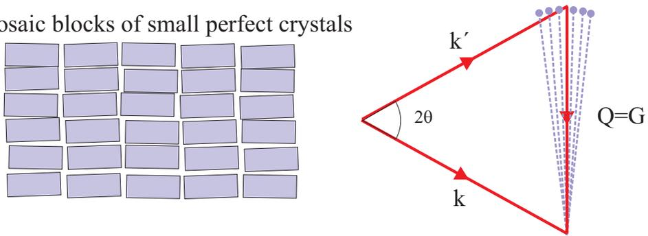
**Fig. 5.19** Left: Real single crystals are often composed of small, ideal crystal grains, also called mosaic blocks which have a narrow distribution of orientations, the so-call mosaic distribution. Right: For a given  $(h, k, l)$  reflection the crystal is rotated, corresponding to rotating  $\mathbf{G}$  about the origin. In this way the integrated intensity from each mosaic block is accumulated.
