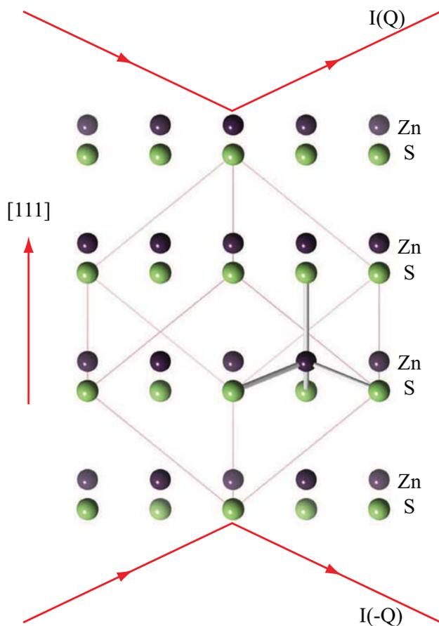
**Fig. 8.8** The magnitude of intensity in symmetric Bragg reflection from a {111} ZnS crystal depends on whether one reflects from the 'Zn' (top) or the 'S' side (bottom). In this way the absolute sense of the polar direction can be determined.
