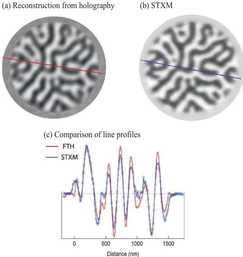
**Fig. 9.26** Comparison of images of the magnetic domain structure in a Co/Pt multilayer obtained with Fourier transform holography (a) and STXM (b). (c) Shows the results of taking a line cut through the images and demonstrates that the two techniques have comparable spatial resolution. (Images courtesy of Joachim Stöhr.)
