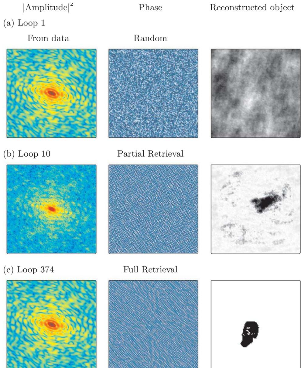
**Fig. 9.22** Numerical example of phase retrieval using an iterative, phase retrieval algorithm that proceeds in a number of loops. The test object and its calculated diffraction pattern are given in Fig. 9.21.
