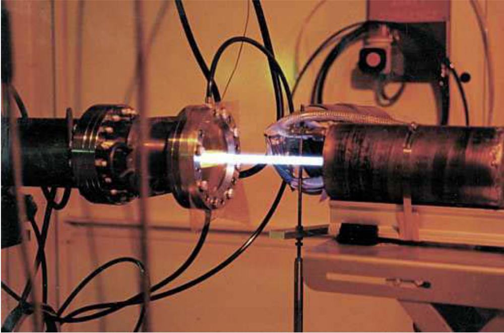
**Fig. 2.15** The white X-ray beam from the wiggler at the ID11 beamline, ESRF. The X-ray beam emerges from an evacuated beam tube with an intensity that is high enough to ionize air. (Image courtesy of Åke Kvick, ESRF.)
