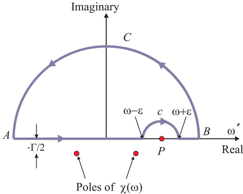
**Fig. 8.3** The Kramers-Kronig relation can be derived from Cauchy's theorem using the contour integral in the complex plane shown here.
