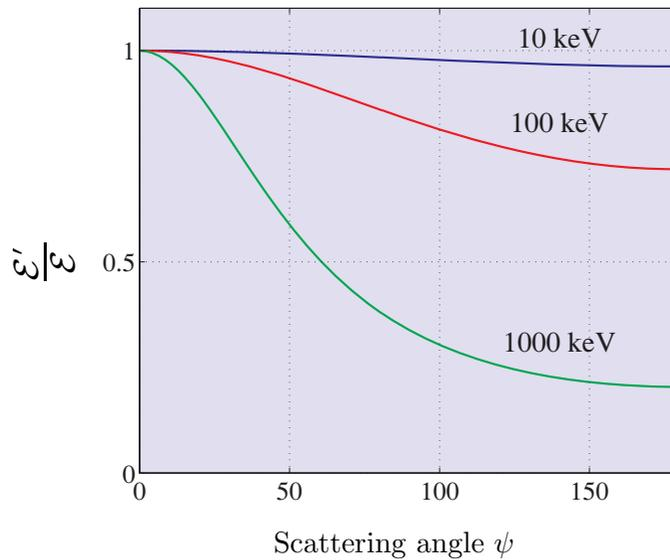
**Fig. 1.10** The ratio of the energy  $\mathcal{E}'$  of the scattered photon to the energy  $\mathcal{E}$  of the incident one as function of scattering angle. The curves have been calculated from Eq. (1.15) with  $\lambda_c k = \mathcal{E}/mc^2 = \mathcal{E}[\text{keV}]/511$ .
