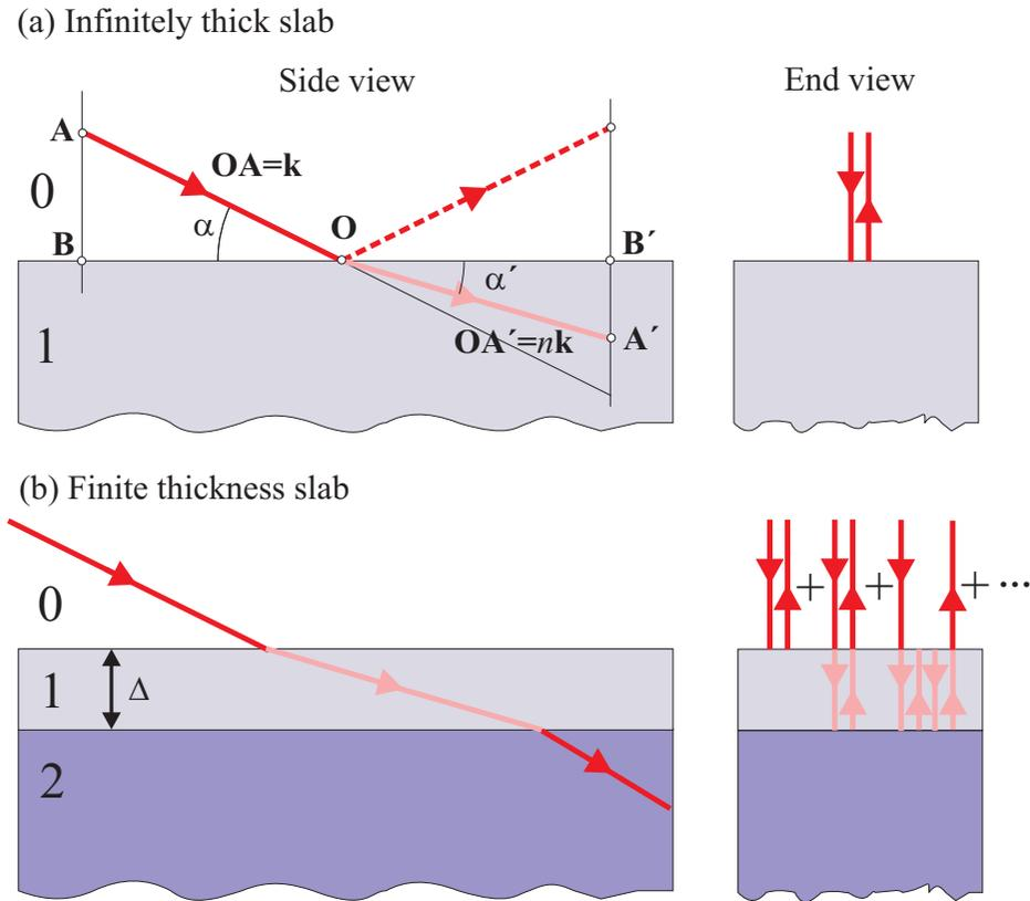
**Fig. 3.6** Reflection and transmission from a slab of infinite (a) and finite (b) thickness. The finite slab is of thickness  $\Delta$  and the total reflectivity is the sum of the infinite number of reflections, as indicated in the right panel of (b).
