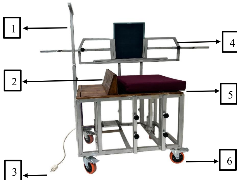
Gambar 4.7 Hasil Rancang Bangun Alat Bantu Pemeriksaan Knee Joint Lateral Stress View
